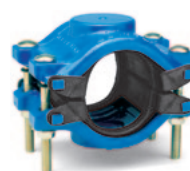
Serie 253 Universal-Schelle DN 80-300 Gas: PN 7 Wasser: PN 16 GJS
